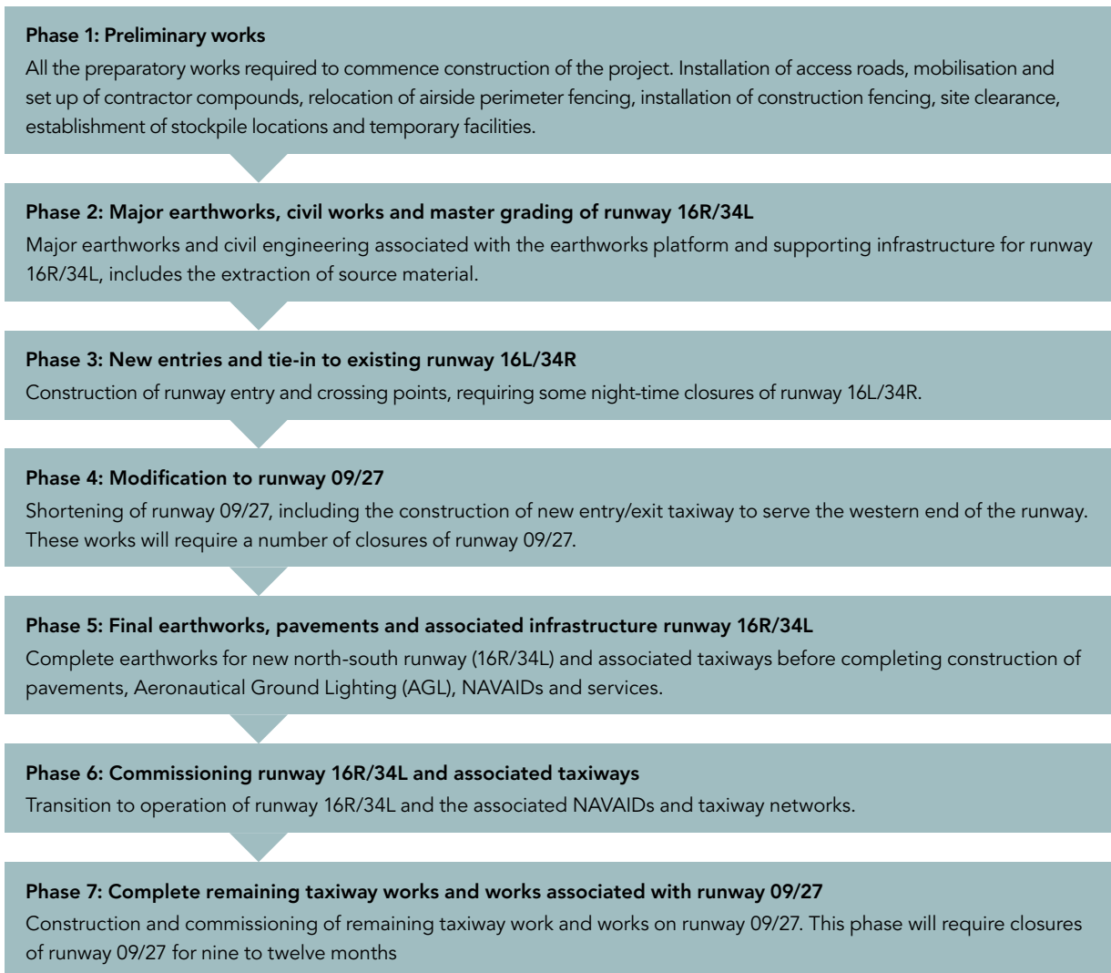
Figure A5.2 Construction phases
