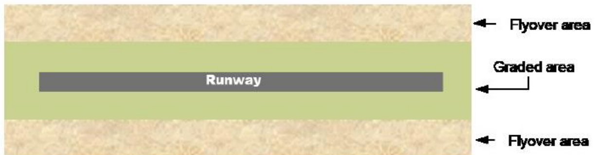
Figure 1: Composition of a runway strip
